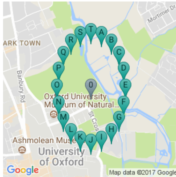
Figure 4.7: Points for cosine-haversine and Vincenty formulae comparison in typical area (different bearing) with point 0 as the centre of the typical area
