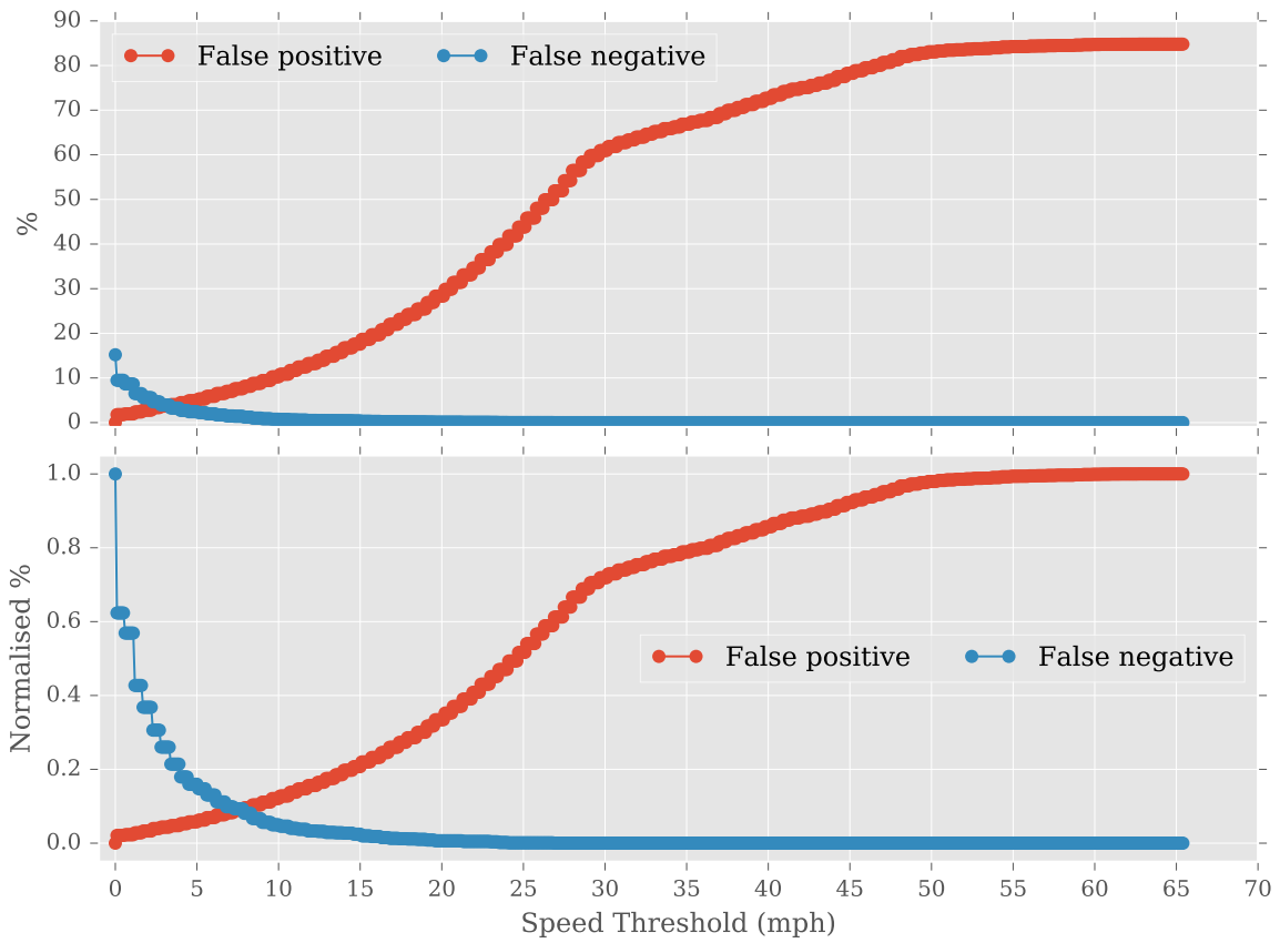
Figure 4.32: Percentage of false positives and false negative for using different speed threshold as halt
