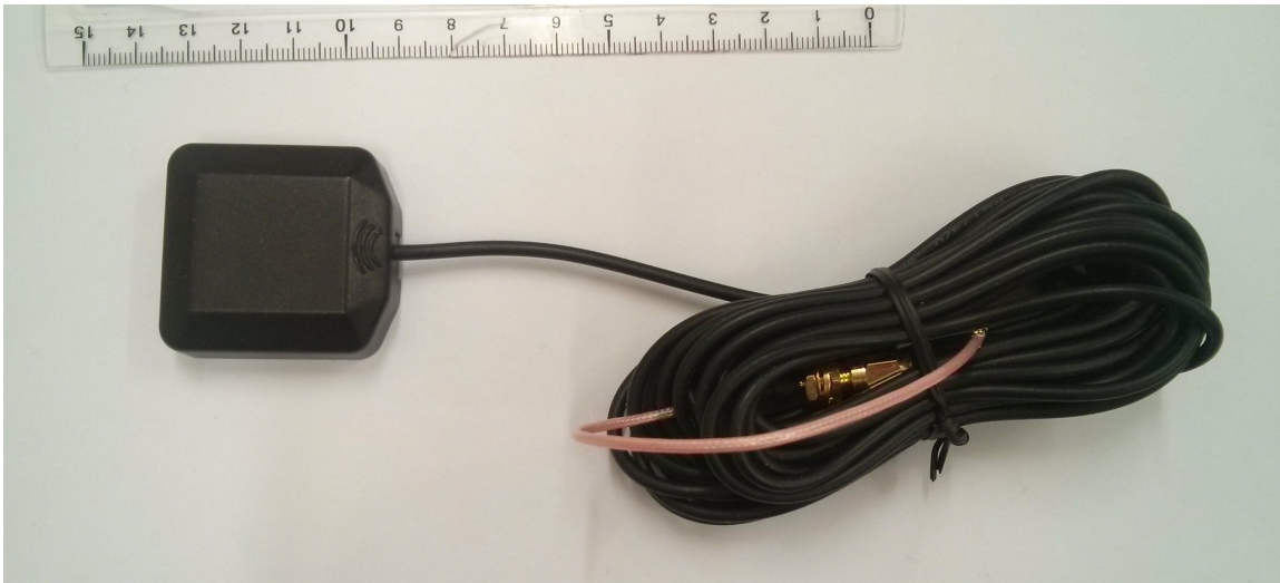
Figure 6.5: Image of external antenna for Adafruit Ultimate GPS HAT
