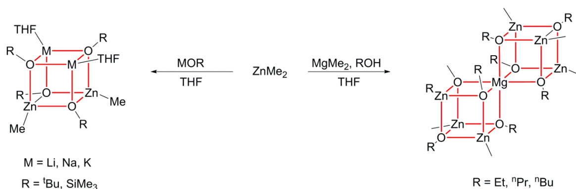
Figure 1.14. The synthesis of bimetallic alkyl zinc heterocubanes, using \text{ZnMe}_2 and the corresponding dopant precursor in THF.
