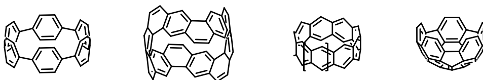
Figure 1.13: Synthesised and proposed CNT segments. From left to right; [6]CPP, carbon nanobelt (Itami, 2008), [ n ]cyclacene (not synthesised), (5,5)CNT end-cap.
