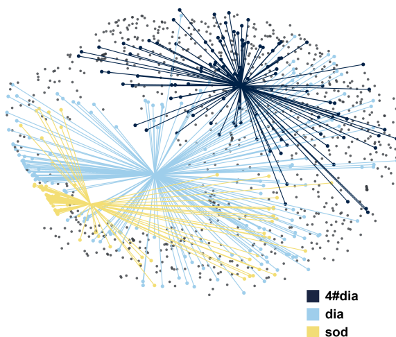
Figure 3.2: Geometric diversity within isorecticular groups of AB_2 MOFs. The graph shows a two-dimensional visualisation of the cg-SOAP-based structural distances using an MDS embedding: generally, the closer two points are, the more similar their coarse-grained and re-scaled geometric structures. The distribution of the three most commonly occurring topologies within the dataset ( dia , sod , and fourfold-interpenetrated dia , denoted 4#dia ) is emphasised by lines that originate from the respective centroid. Dataset entries with different topologies than the three aforementioned ones are all represented by grey points.
