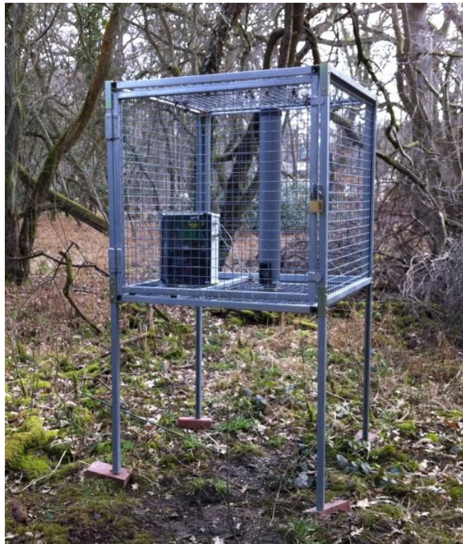
Fig. 2. Feeding station containing an automated data logger and feeder with grey sleeve and two black RFID antennas (one visible) in front of seed access holes. A motor moves the sleeve up two inches to open the feeder and down to close the feeder. All equipment is housed in a squirrel-proof metal cage which allows access to small birds through the mesh.
