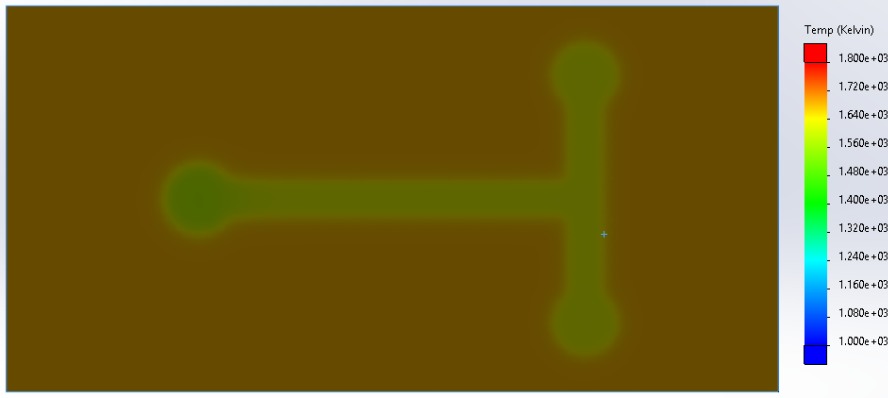
Figure 6.7: Temperature distribution in the insert configuration with Tungsten insert and Inconel 718 base plate.
