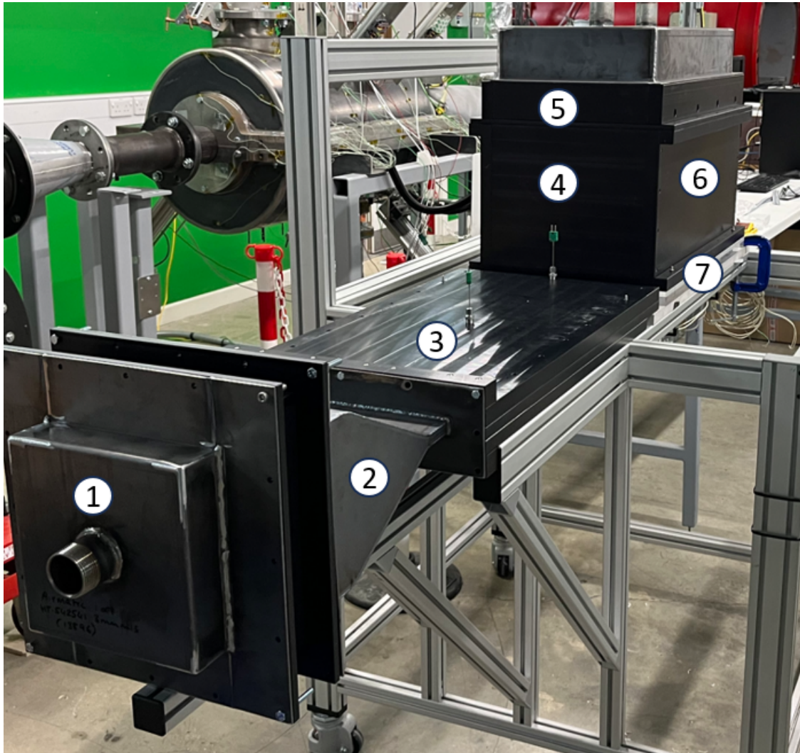
Figure 4.2: Annotated photograph of the assembled experimental apparatus. Key components are indicated with numbered callouts: (1) Crossflow inlet plenum, (2) Crossflow converging nozzle, (3) Crossflow channel, (4) Main jet plenum, (5) Jet inlet flow-straightener cassette, (6) As-built vortex tube inlet location (side-mounted), and (7) Heated working section.
