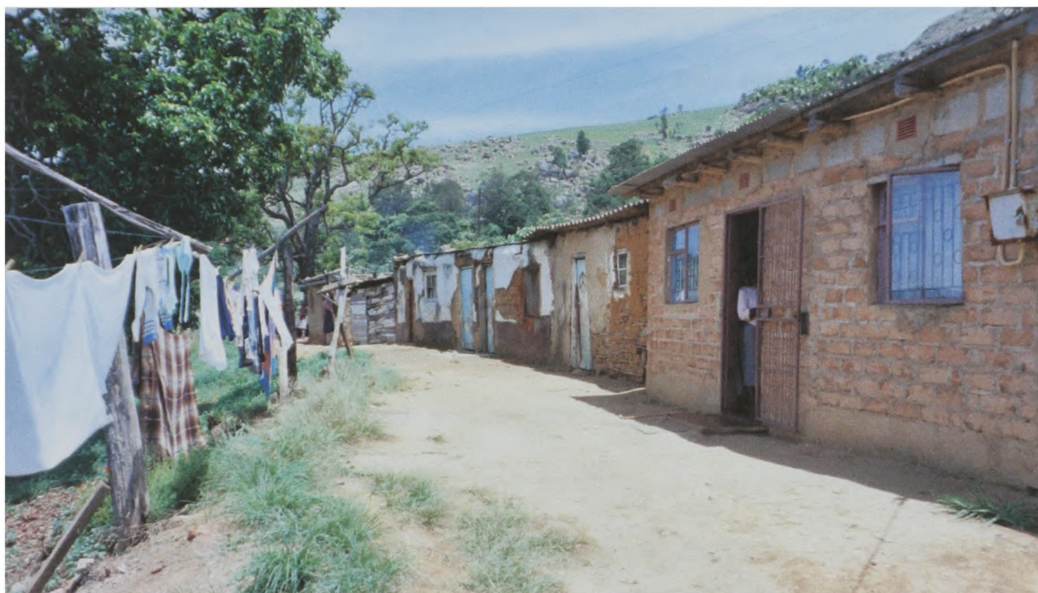
Figure 6: Heterogeneous housing within the informal settlements of Mbabane. Some housing was of brick construction with sanitation and electricity, as in the foreground. Other housing was constructed of mud and wattle and lacked services or vegetable plots.
