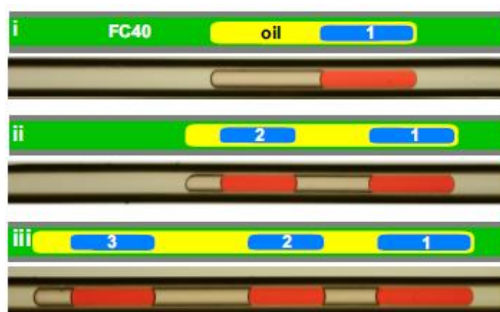
Figure S1. Trains with 1, 2 and 3 carriages. Schematics (with micrographs below) of tubes containing carrier fluid (FC40) surrounding a ~10-nl oil super-drop (tetradecane + 1% Span 80) engulfing 1-3 10-nl aqueous drops (the carriages in a train) containing red dye. A 150- \mu m tube was loaded by dipping it successively into wells containing: (i) carrier fluid (FC40), water, oil, water, and FC40, (ii) FC40, water, oil, water, oil, and FC40, and (iii) FC40, water, oil, water, oil, water, oil, and FC40. Fluid was drawn into the tube (0.05 ml/h) only when dipped below the surface of the fluid.
