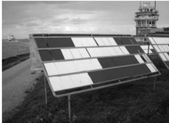
Figure 2.10 - Typical setup for outdoor exposure of coated panels [71]
