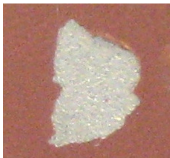
Figure 4.65 - Image of area underneath a blister on a PCE coating exposed to NaCl solution (size 5mm x 5mm)
