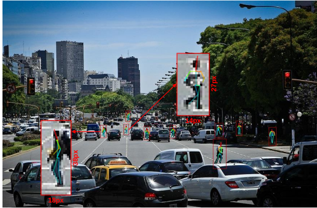
Fig. 1. Human pose estimation at a distance. Given a small low-resolution patch of an image (detected by [13]), the proposed method estimates the joint probability distribution of all body parts, despite individual pixels’ noise and ambiguities. Image taken from the Tiny People dataset
