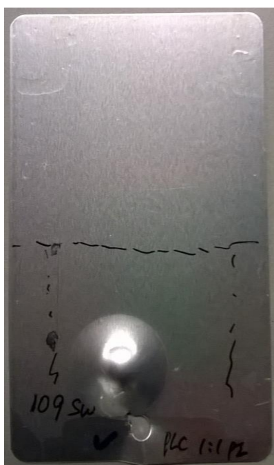
Figure 6. 8 – Picture of coating material after delamination (PLC:TMPSH = 1:1).
