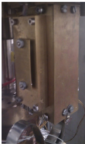
Figure 6.6 - The box used to shield the lower levels from the 100K radiation. This is also wrapped in aluminium foil for extra protection.
