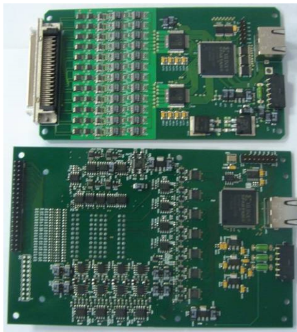
Figure 3.1 - The 12 Channel DAQ board (top) and the Pre-amplifier and Bias control board (bottom) used in the electronics chain at room temperature.
