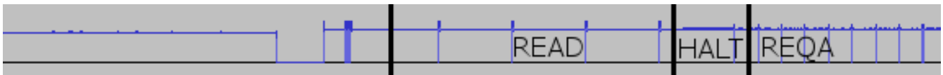
Figure 13. Signal Received with Fixed Tag and Arduino Reset: PICC (PCD) Transmissions Above (Below) the Average
