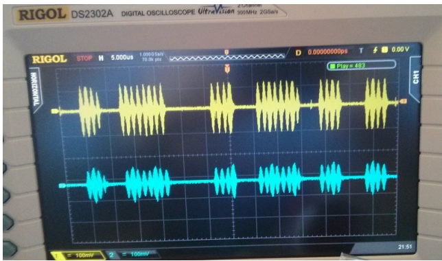
Figure 19. Tag TX in Yellow, RC522 Antenna in Blue
