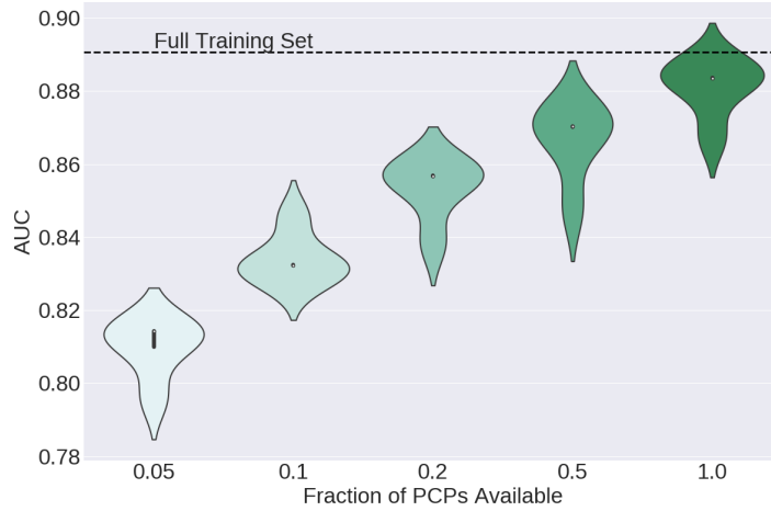
Figure 6.6: AUC of SVM model trained on a fraction, F , of the PCPs and evaluated on a held-out set of data. Results are averaged across five random seeds. The horizontal dashed line depicts the performance of an SVM trained on all instances ( N = 76644 ) in the training set. We show that PCPs are effective dataset distillers; despite a 12-fold reduction in the number of training instances ( F = 1 , \Omega_{train} = 6,387 ), the SVM achieved similar performance (AUC \approx 0.89 ) to one trained on all instances.
