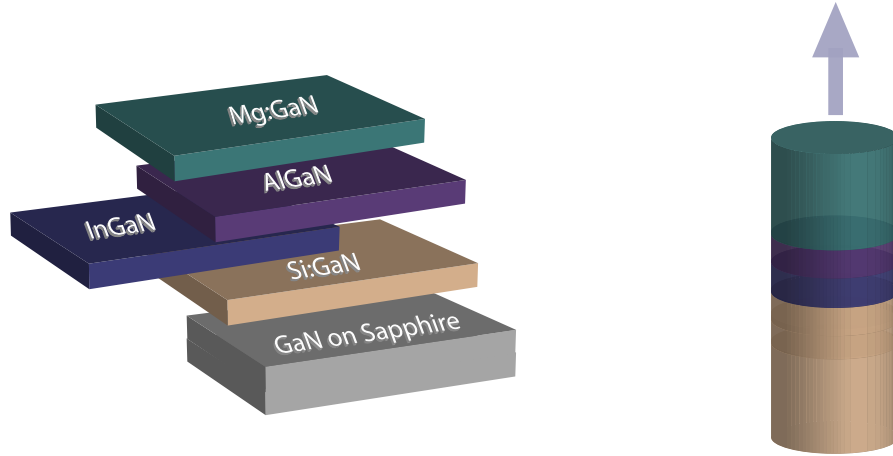
Figure 6.1: - Diagram showing the bespoke LED with a exploded view showing the different layers. On etching, this results in nanorods with structure shown on the right.
