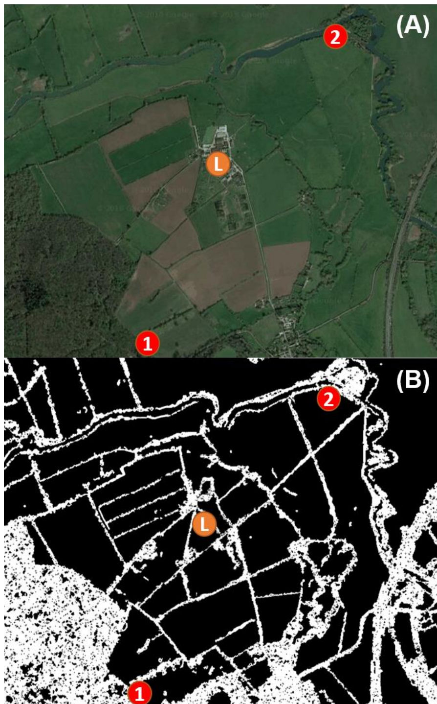
Figure 2.4 — Linear Feature detection method. Canny edge detection of an aerial image (A) to produce a binary image (B) of the flight area. Release sites 1 (Wytham Hill) and 2 (Kings Mill Lock) are labelled along with the home loft 'L'.
