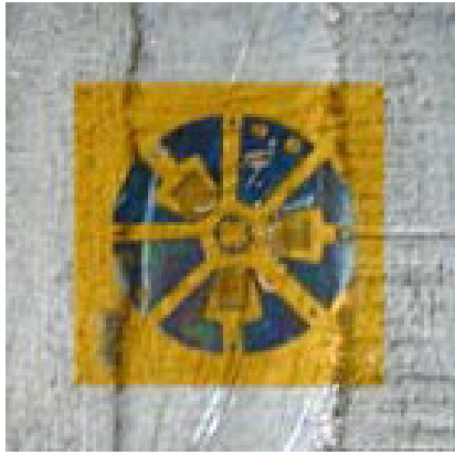
Figure 1.3: An illustration of a 45° strain gauge rosette on an Electron Beam (EB) weld sample [8]
