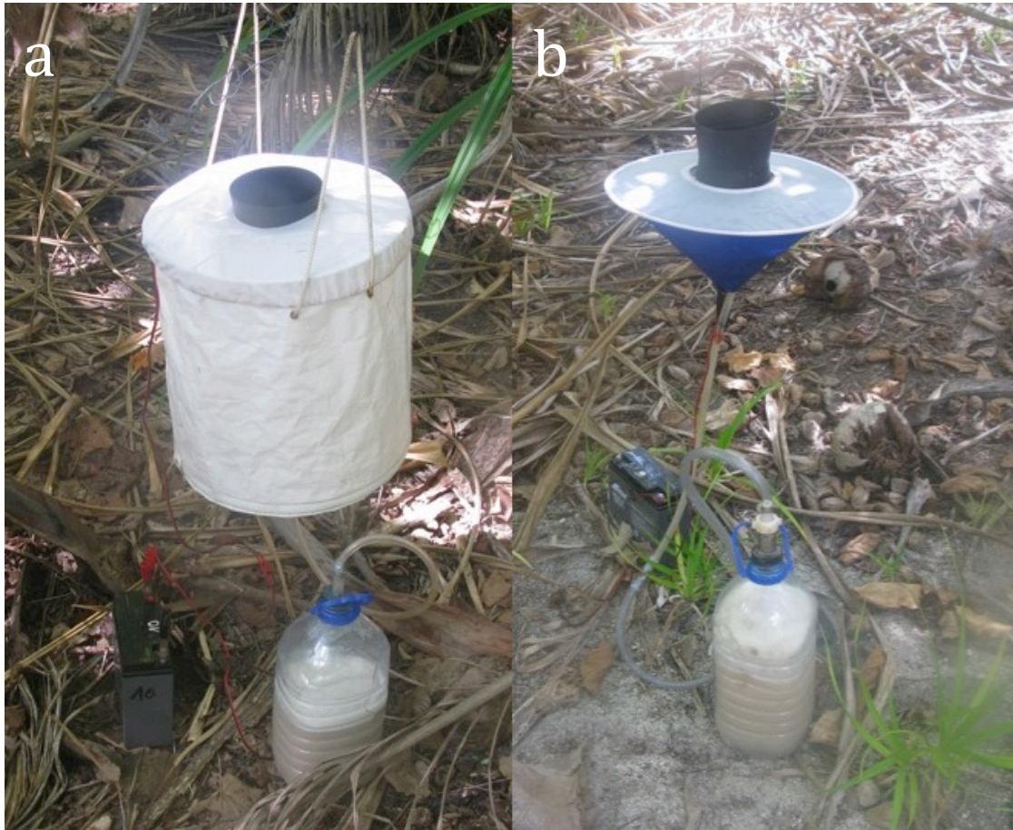
Figure 3.4. BG Sentinel and BG Mosquito trap connected to 12V battery. CO 2 was produced using 5L bottle containing a mixture of yeast, sugar and water.
