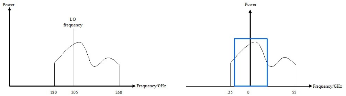
Figure 1.9: Sketch of (left) the input signal spectrum into the telescope with the position of the LO marked and (right) IF band. The blue square shows the area selected by a bandpass filter in the IF.
