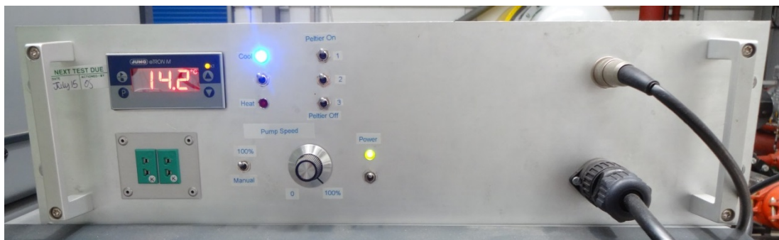
Figure 6.6. Wall heater/cooler hardware.
