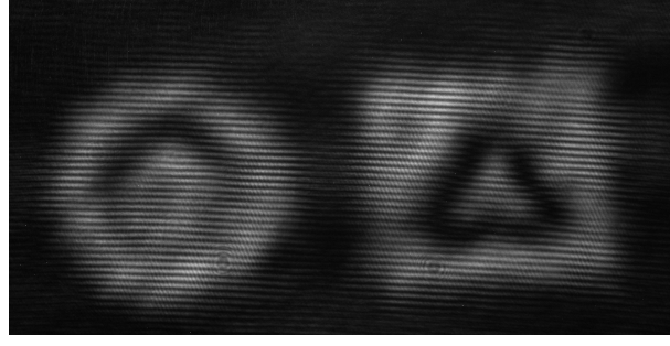
Figure 10.8: Raw phase measurement data with the interferometry arm unblocked.
