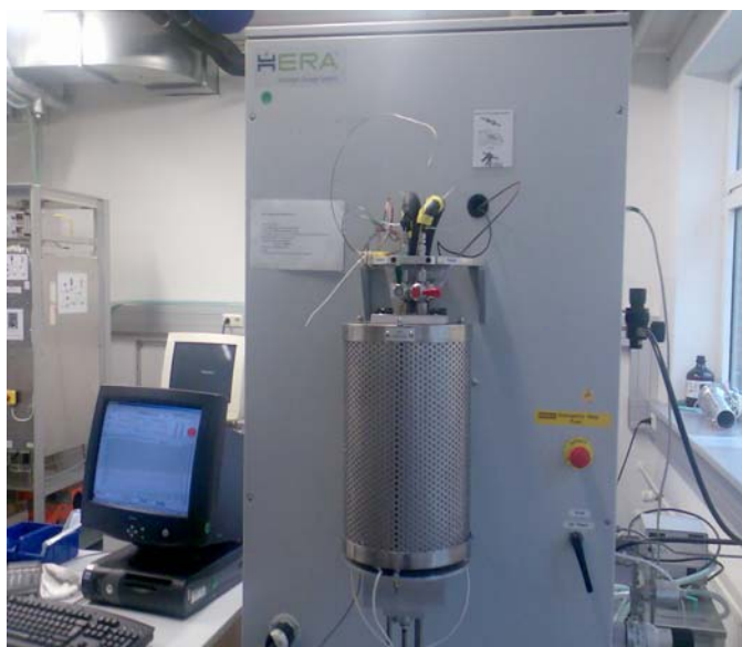
Figure 3.4: Photograph of the C2-3000 Sievert's-type apparatus used for volumetric analysis at GKSS Research Center, Geesthacht Germany.
