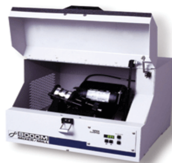
Figure 3.1: Photograph of a SPEX 8000M shaker mill at GKSS Research Center, Geesthacht Germany.
