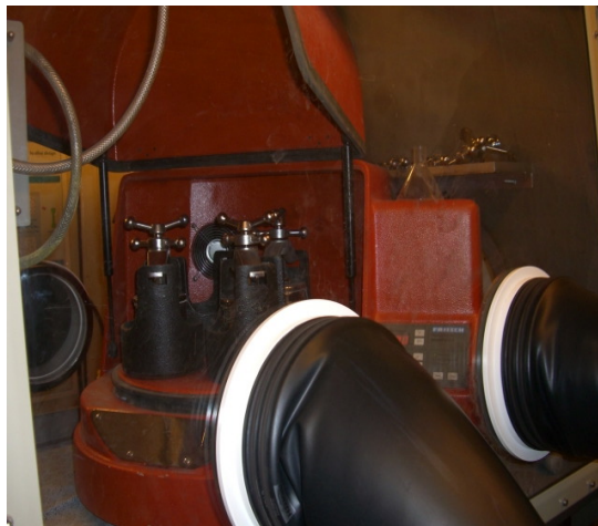
Figure 3.2: Photograph of a Fritsch P5-planetary ball mill at GKSS Research Center, Geesthacht Germany.
