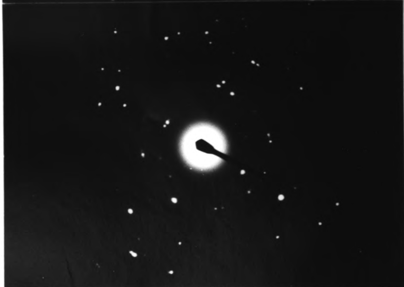
Fig.7-7 Typical SAED patterns from the oxide films removed from amorphous \text{Fe}_{40}\text{Ni}_{40}\text{B}_{20} (a) after 140h oxidation at 350^{\circ}\text{C} and (b) after 500h oxidation at 350^{\circ}\text{C} .
