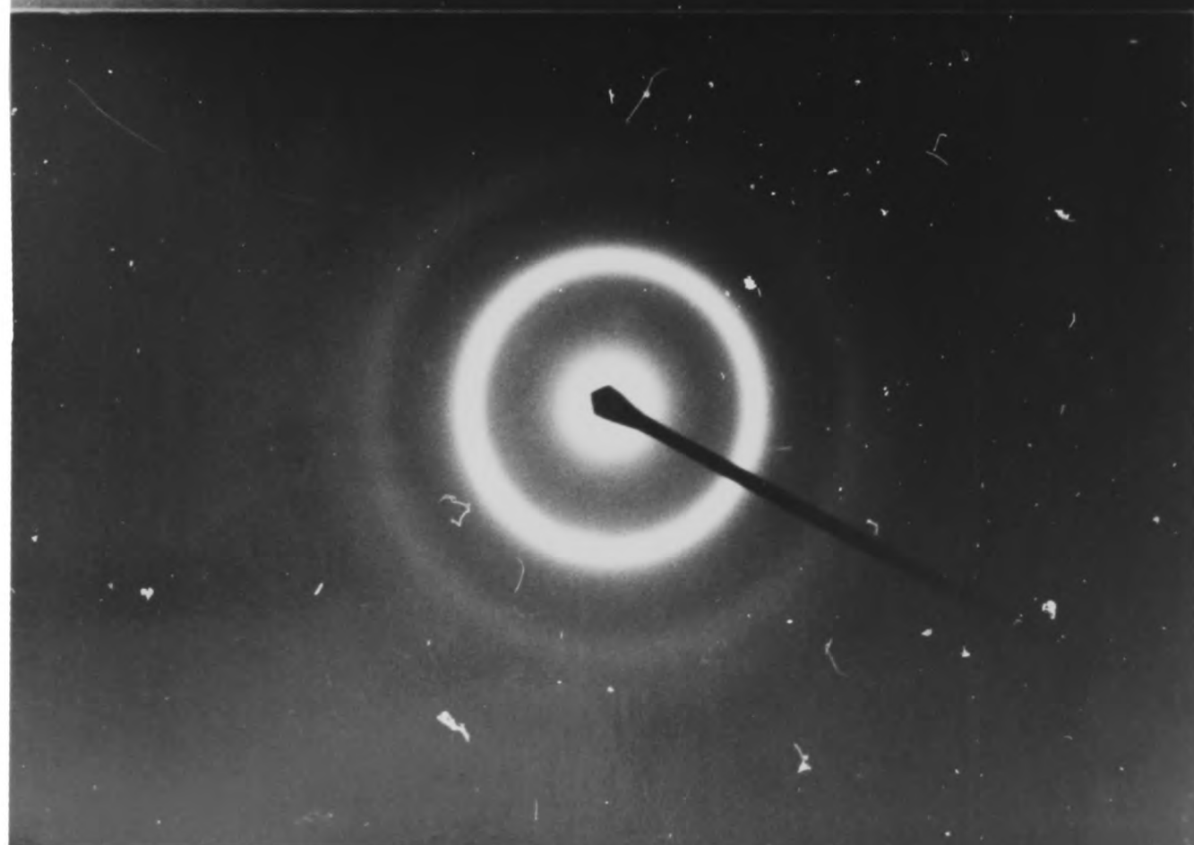
Fig.4-11: TEM micrographs of unoxidised amorphous Fe 40 Ni 40 P 14 B 6 foils; (a) bright field image, (b) SAED pattern.
