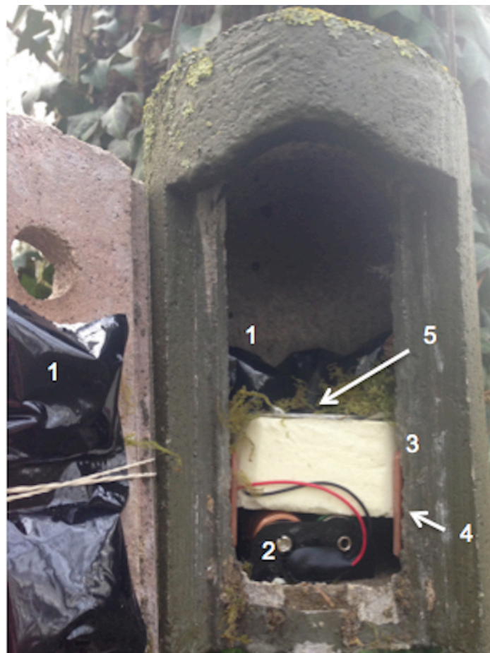
Figure 3.2: Photograph of experimental set up for a heated box. Key components of the set up are numbered 1) Ice packs mounted front and back of the box, 2) battery pack, 3) polystyrene insert, 4) plastic ring to hold polystyrene above the battery pack, 5) metal disc topping the bulb. In control and cooled boxes the battery pack would be replaced by a second polystyrene insert.
