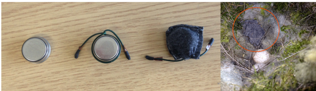
Figure S2.1: Photographs of the construction of in-nest iButtons. From left to right: the iButton alone, the iButton with its garden wire anchor, the iButton secured in cloth pouch, the finished iButton placed in a nest amongst the eggs
