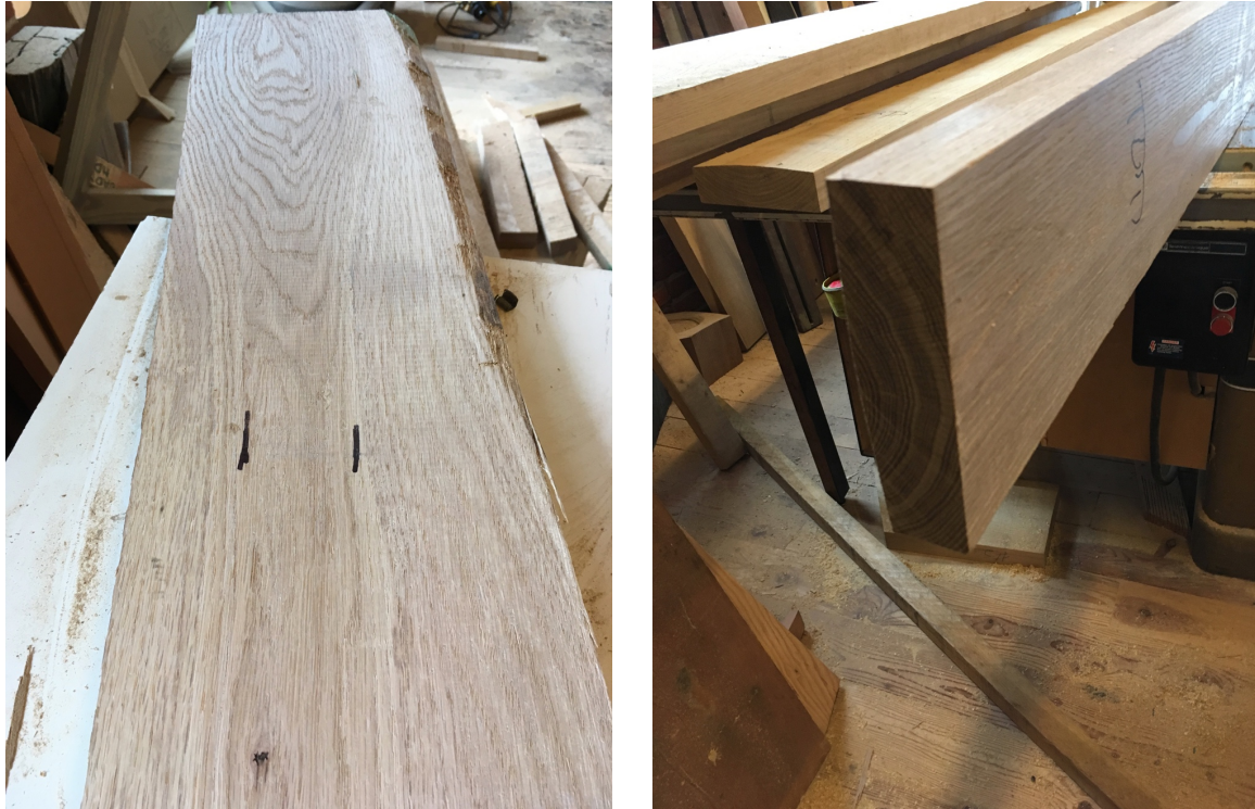
Figure 33: A stripe of heartwood between two marker lines (left); the end-grain, another visual clue (right)
