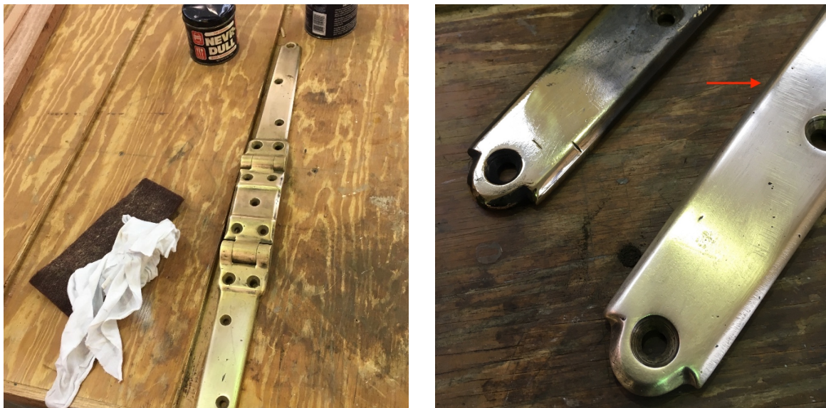
Figure 20: A hinge after polishing (left); close-up of marks from an electric grinder (right, at arrow)
