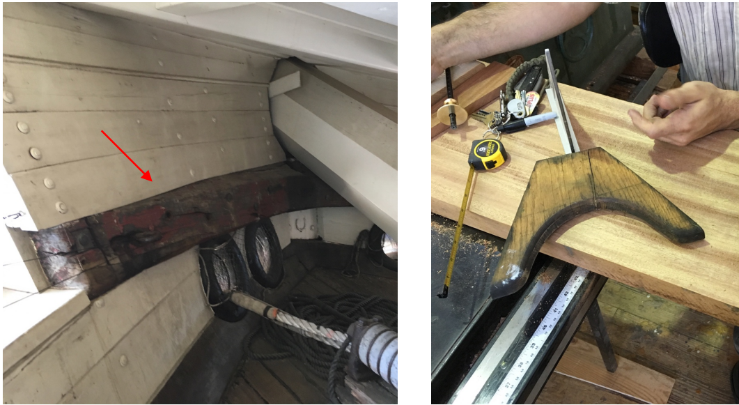
Figure 8: The breast-hook on Integrity (left, at arrow) versus one from a Riverside rowboat (right)
