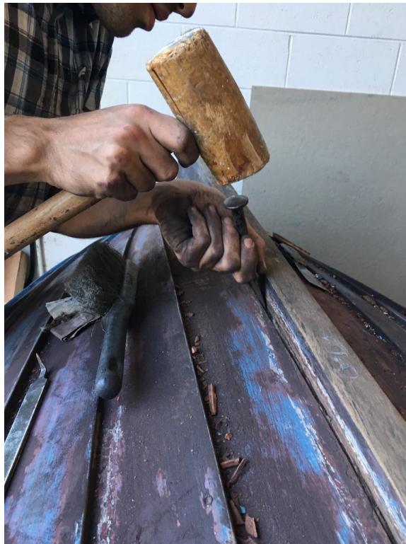
Figure 48: Chris installed cotton caulking on a rowboat while I scraped away old paint
