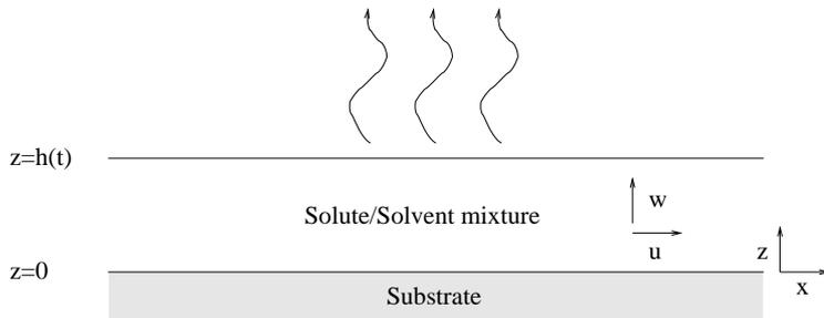
FIG. 2.1. Sketch of the physical situation with a thin liquid layer consisting of a mixture of a volatile solvent and a non-volatile polymer.
