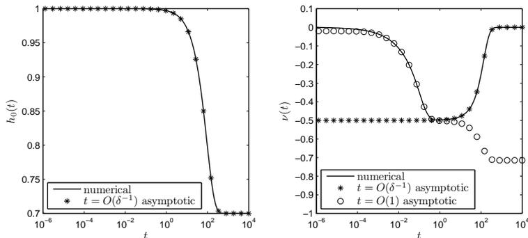
FIG. 3.1. Comparison of the asymptotic approximations (correct to  $O(\delta)$ ) with numerical solutions of the base state for the full one dimensional equations (3.1). The film thickness is shown in the left and the average concentration gradient (explained in the text) in the right figure. Note that the leading order for  $h_0$  for  $t = O(1)$  is trivial and has therefore been omitted on the left.
