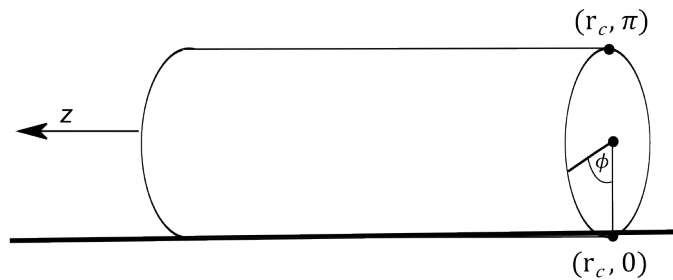
Figure 9.3: A scheme of the ‘Cylinder on its side’ and the relevant points for one-dimensional (1D) diffusion model.
