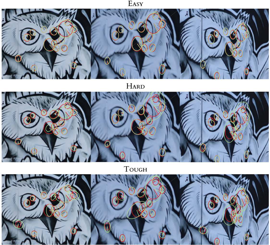
Figure 4.4: Example of the reprojected detections with a generated geometry noise on three images of a single sequence, visualized with the detected regions for the EASY, HARD and TOUGH distributions in each row respectively. Red ellipses are reprojected detections from the reference image using the ground truth homography H_{gt} for a given image in a sequence. Green ellipses are ellipses with additional geometry noise of a given category. See fig. 4.5 for the extracted patches.
