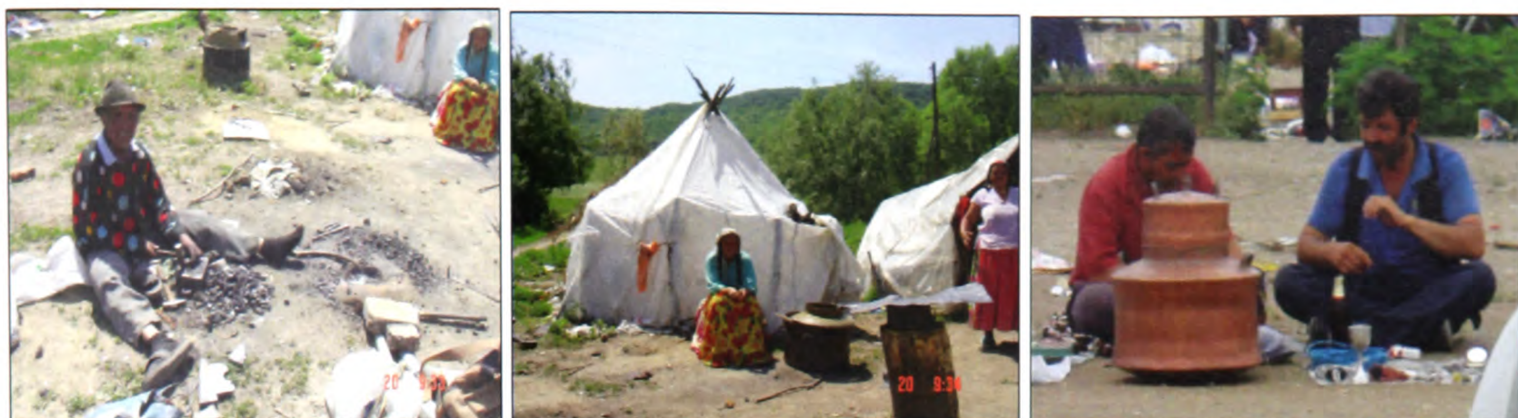
Figure IV.2 Caldarari Gypsies in Transylvania in the process of melting down scrap copper, welding copper sheets into copper stills and selling the finite product at the local market.
