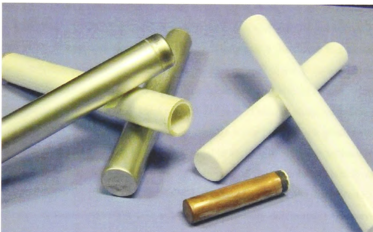
Figure 3.1: A selection of Johnson Matthey membranes. The large tubes are 200 mm in length and 25 mm in diameter. The white tubes (right) are the bare sol-gelled tubes. The silvery tubes have a Pd/Ag membrane. The small tube has a Pd/Cu membrane (Johnson Matthey, 2001).
