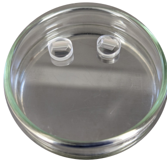
Figure 2.3: The lenses used in an SFB experiment, after the silvered mica has been cut to size, removed from the base sheet and then glued onto the glass lens, silver side down.
