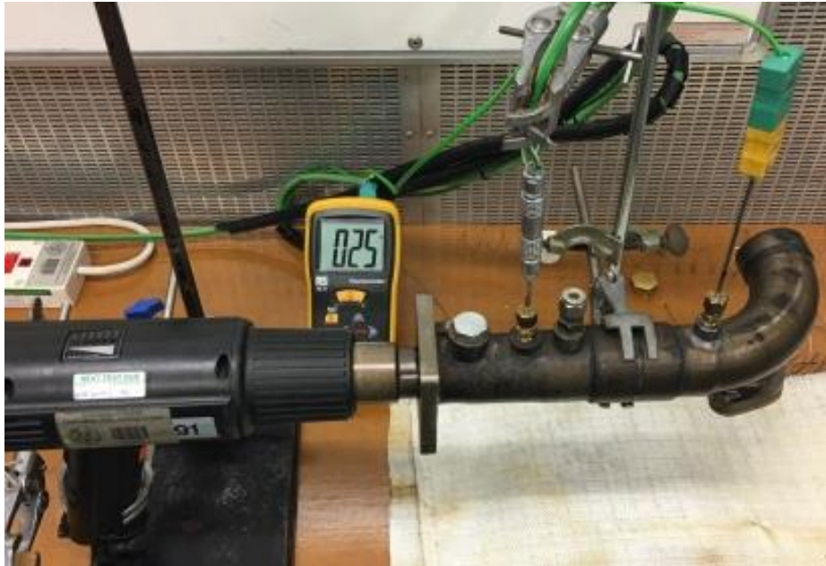
Figure 5.3: Test bench installation using the exhaust manifold and a heat gun as a heat source. The installation of the 3TC-probe and the reference thermocouple are identical to the engine installation.
