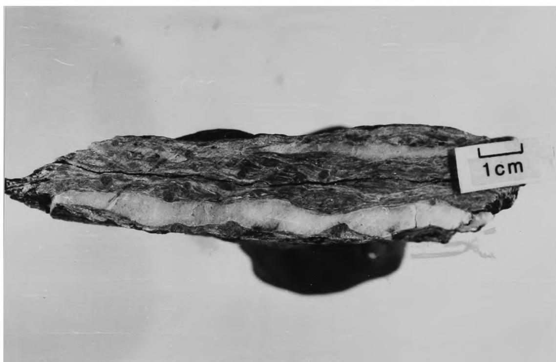
Fig.3.4b. Sectioned Ds tectonite showing undulating aspect of Ss due to movement along eccs. The displacements are shown clearly by the offset of the layer of vein quartz. Bl29, area 1.
