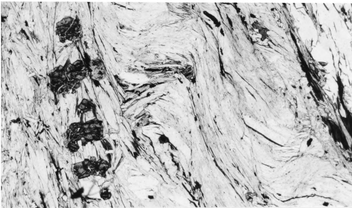
Fig.3.12. Deformed quartz showing undulose extinction and sutured grain boundaries indicative of crystal plastic processes. The mesoscopic Ss foliation is defined by the preferred orientation of platy minerals. The obliquity of the quartz grain-shape fabric suggests a top to NW sense of shear. K5, area 1, crossed nicols with a sensitive tint plate.
