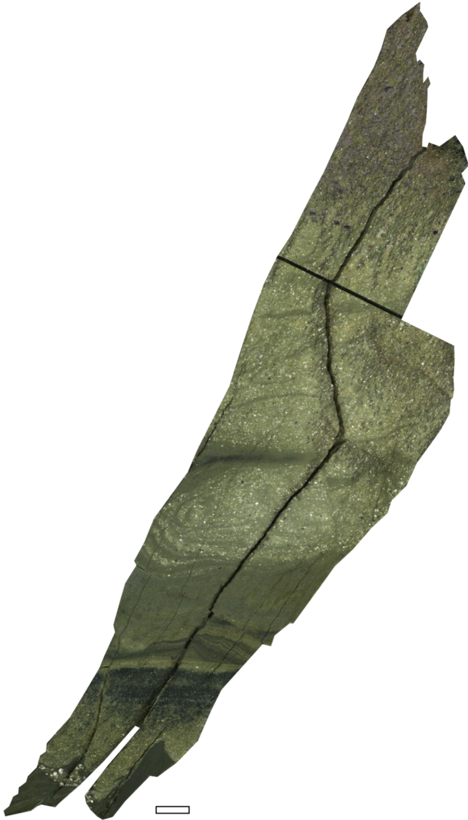
FIGURE 3.5. Slabbed section of the SH-2 geochronological sample, from the Fermeuse Formation. The slab shows disturbed bedding within a light green tuffite, thought to have been at the base of a slump. The top section of the slab had been stained for carbonate (red, blues, and purples) using Alizarin Red-S and Potassium Ferricyanide. Scale bare is 1 cm.
