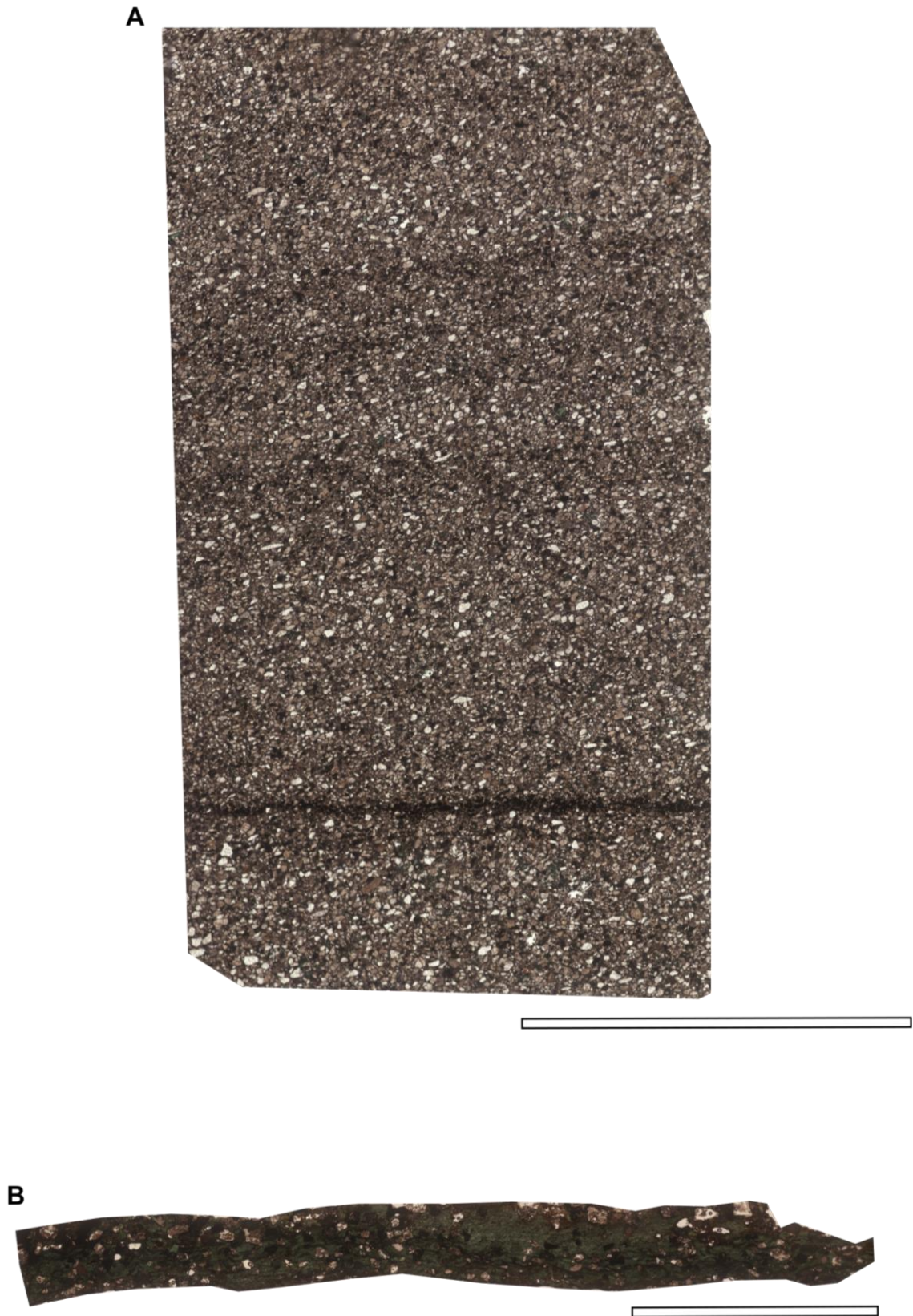
FIGURE 2.15. Thin sections from the Mistaken Point Formation. A) Cross-laminated sandstone from between the 'D' and 'E' Surfaces at Mistaken Point. B) Chloritic crystal-tuff that lies directly upon the fossiliferous 'E' Surface. Scale bars are 1 cm.
