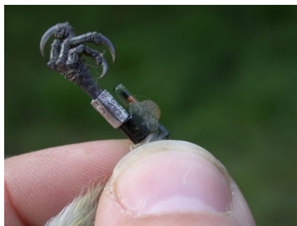
Figure 5.5: Birds are “ringed” with a harmless RFID device that generates a sensor observation when the bird comes into proximity of the logger-enabled feeders placed across Wytham Woods, Oxfordshire. Photo credited to Edward Grey Institute and used with permission.
