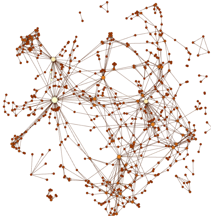
Figure 9.3: The network of the network analysis software used in this thesis. The N = 575 nodes represent MATLAB scripts and the M = 1085 links represent calls from one scripts to another. The size of each node expresses its in-degree and its brightness corresponds to its PageRank centrality.
