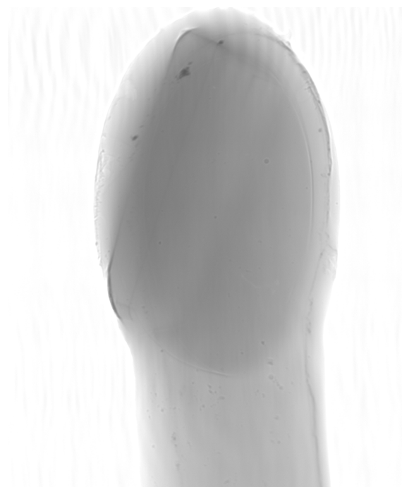
Figure 1.3: Flat-field corrected projection images of Thermolysin. The crystal is glued on the mounting loop by mother liquor.
