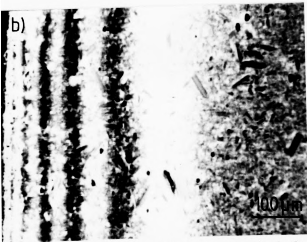
Fig. 7.11 Acoustic images a) at focus, and b) at a defocus of -13\mu\text{m} , of specimen 23. The obelisks have increased in size, and some are visible at focus.
