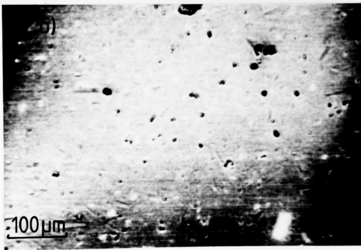
Fig. 7.13 Acoustic images a) at focus, and b) at a defocus of -12\ \mu\text{m} of cycled electrolyte tube (635 cycles) after storage under a thin carbon film. Obelisks can be seen but do not appear to have increased in size.
