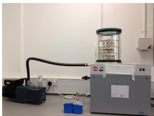
Figure 3.6: One mL freeze dry stocks being made in the mini Lyotrap machine
