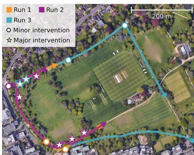
Fig. 9 Kilometer-scale navigation: We deployed our system to learn to segment the footpath of a park after training for a few steps. We executed 3 runs starting from different points in the park: orange filled square run 1 (0.55 km), purple filled square run 2 (0.5 km), and blue
