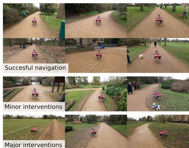
filled square run 3 (1.4 km). Minor interventions were applied to guide the robot in intersections; major interventions (★) were required for some areas when the robot miss-classified muddy patches for the path
