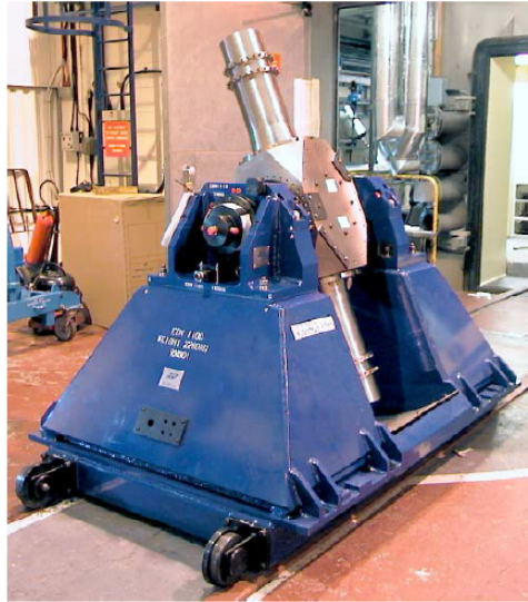
Figure 3.1: Photo of the Rolls-Royce rotating heat transfer rig [97]
