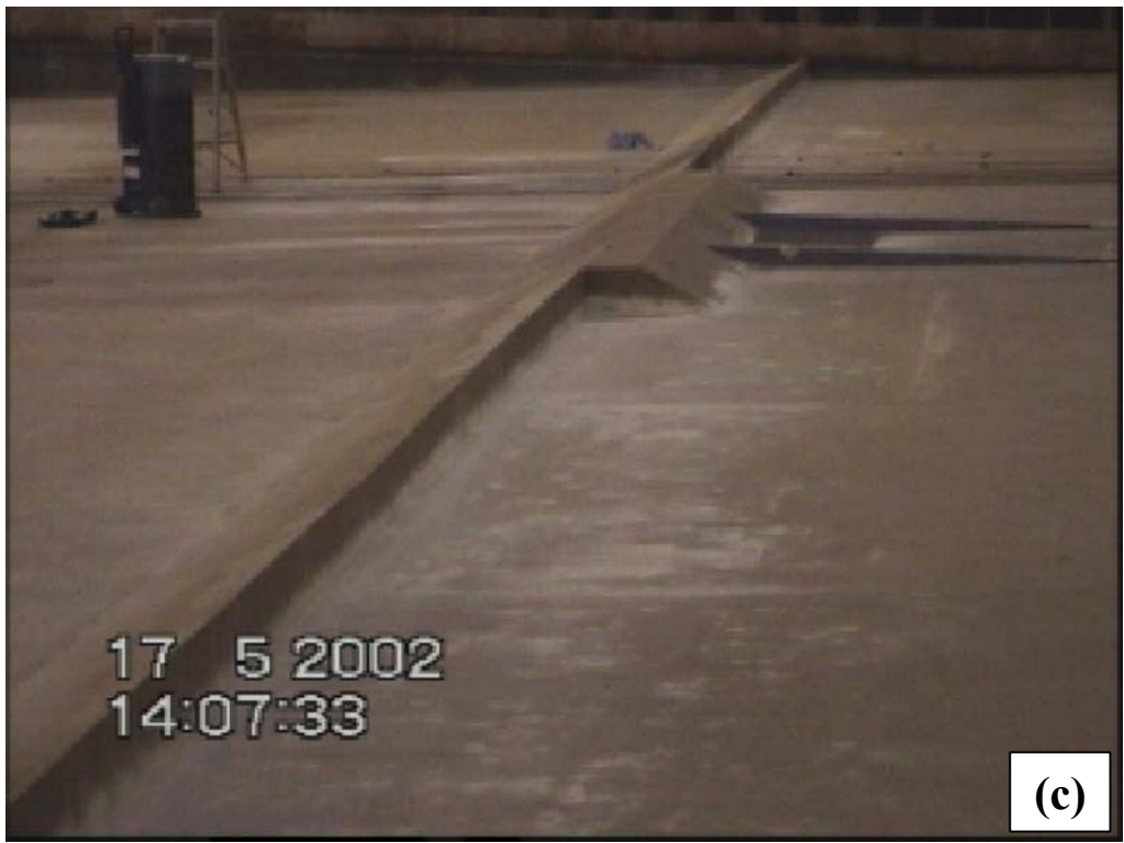
Figure 4.19: Sea wall constructed in the UKCRF. (a) Dimensions of the sea wall. (b) Location of the sea wall relative to the toe of the beach. (c) Sea wall in the dry basin showing full central section and sloping front face of remaining sections.
