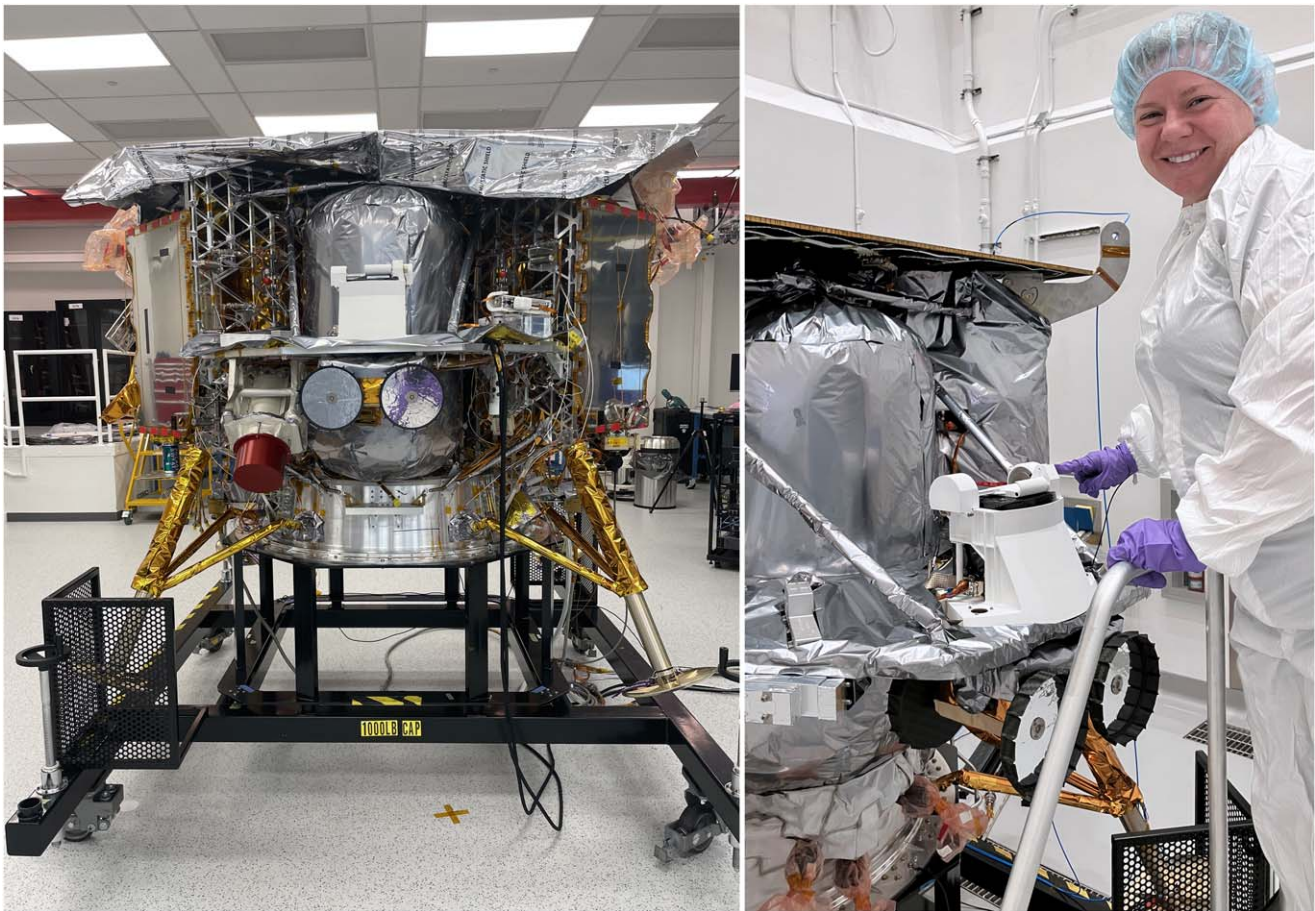
Figure 2. PITMS mounted to the Peregrine lander Deck D (left) in the Astrobotic clean room and (right) during remove-before-flight activities (with B.A.C. for scale). The Iris rover (N. Potter 2023) is mounted to the underside of Deck D. The PITMS aperture opens to the +X direction of the spacecraft.
