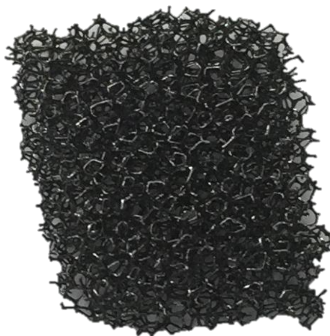
Figure 3.4: Vitreous carbon foam material used in the experiment.
