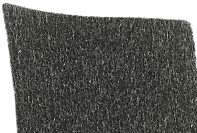
Figure 3.3: The graphite felt material used in this thesis.
