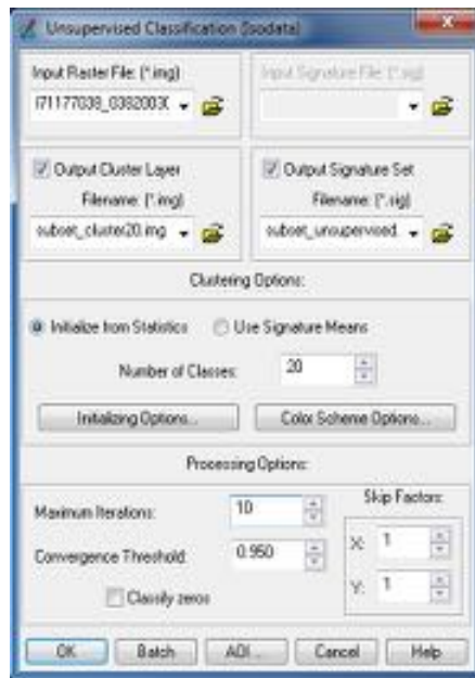
Fig. 4.16: Performing an unsupervised classification using the ISODATA algorithm in ERDAS IMAGINE
