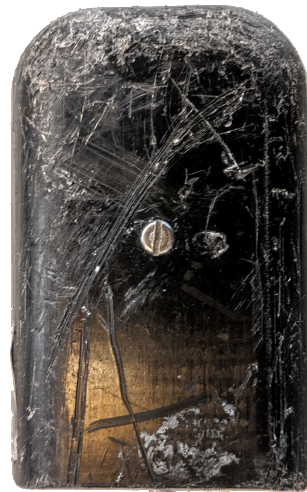
Figure 5.6: A SnapperGPS enclosure after being deployed on a loggerhead sea turtle for two weeks.
