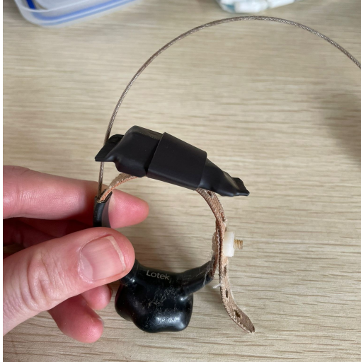
Figure 5.14: A custom collar with a SnapperGPS tag and a VHF transmitter. Credit: Kim Lewandowski Figure 5.15: A woylie carrying the collar. Credit: Kim Lewandowski
