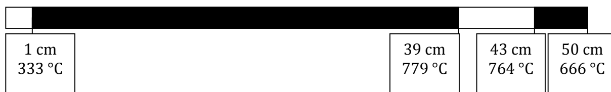
Figure 44. Schematic of what the Kanthal wire looked like to the naked eye after the experiment.
