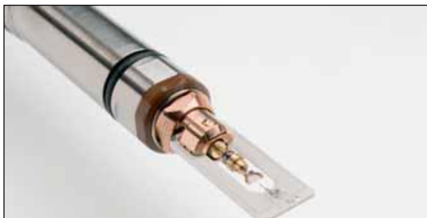
Figure 26. NanoFactory TEM holder used to test the field emission properties of individual CNTs.
