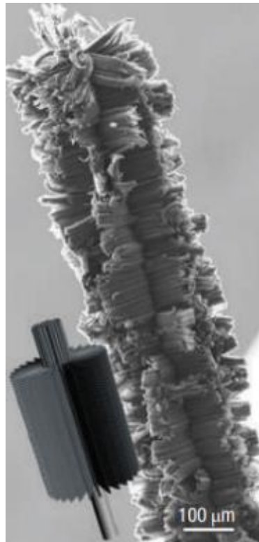
Figure 36. SEM micrograph of CNTs “ridges” on 50 \mu\text{m} diameter Inconel wire. A schematic is inset showing the brush type structure. Taken from [125].
