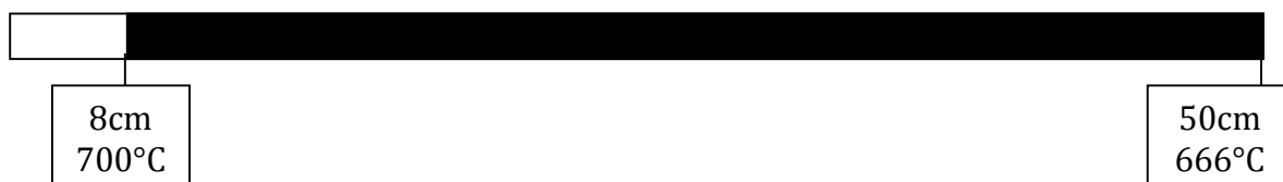
Figure 60. Schematic of the deposit found on the Kanthal wire after growth of N-doped CNTs.
