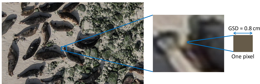
FIGURE B1 Ground sampling distance (GSD) is a measure of the resolution of an image, representing the true distance between the centre of two adjacent pixels. Therefore, if each pixel represents 0.8 \text{ cm} in real life, the GSD of the image is 0.8 \text{ cm px}^{-1} . A GSD of 0.8 \text{ cm px}^{-1} is illustrated here, with the width of each pixel representing 0.8 \text{ cm} in real life.
