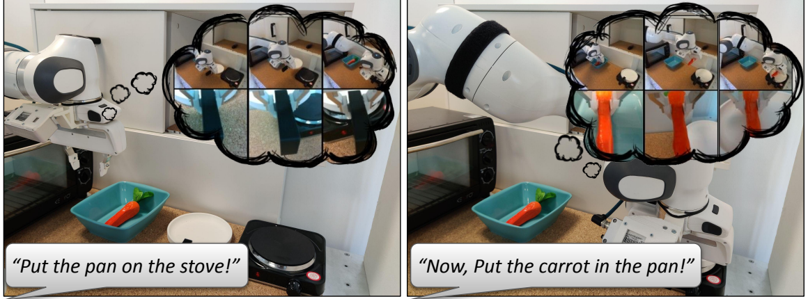
Figure 4.1: LUMOS learns a general-purpose 7-DoF language-conditioned visuomotor policy within the latent space of a learned world model. By optimizing for an intrinsic reward aimed at matching the expert performance within the world model, it effectively recovers from its own mistakes across multiple time steps and reduces covariate shift. Consequently, LUMOS can accomplish complex, multi-tier, long-horizon robot manipulation tasks based on abstract natural language instructions in real-world scenarios, without requiring online learning or fine-tuning.
