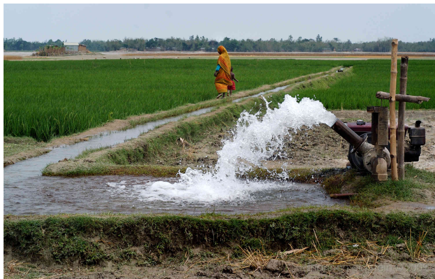
Figure 1.3: Typical configuration of a shallow tubewell with powered pump used for irrigation of rice paddies in Bangladesh..
