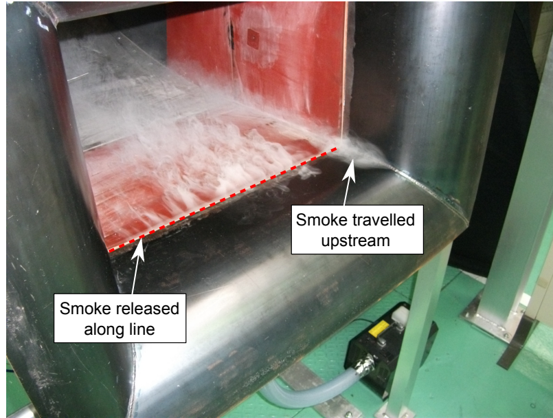
Figure B.1: Smoke flow visualisation in initial inlet
